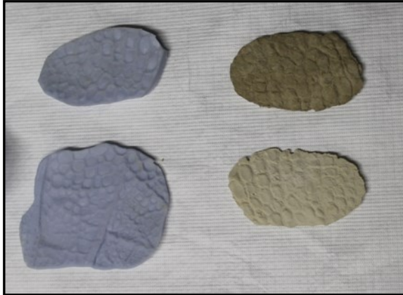
Figure 5. Steramould moulds of skin (left) with moulded test pieces in plaster and papier mâché (right). © Anastasia van Gaver, 2017.
