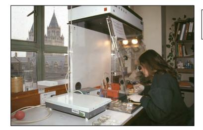
Fig. 1 Hazardous chemicals such as glacial acetic acid, phenol and xylene require the use of a portable fume hood.
