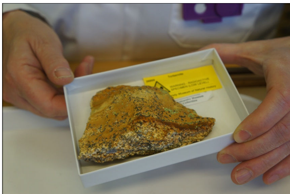
Fig.3. Distance can be increased by picking up a specimen's card tray rather than the specimen itself. (photo: Simon Haycox, University of Oxford)
