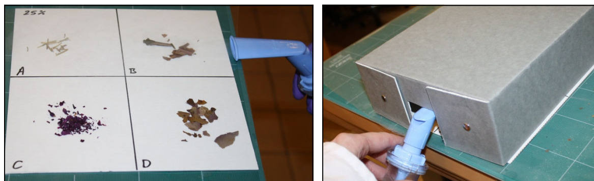
Fig. 3. (left) Consolidant cloud creation using a nebuliser. (right) Make-shift enclosure to prevent cloud dispersal.
