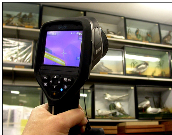
Fig. 1. An example of an infrared thermal imaging camera: The author's 'FLIR E40bx' in use. Image resolution 160 × 120 pixels (providing 19,200 data points); digital infrared still images and video; range minus 20°C to plus 120 °C; thermal sensitivity <0.045 °C; built-in 'normal' digital camera (3.1 megapixels); one LED spotlight; and wireless/Bluetooth technology.
